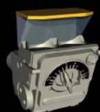
Q32247 Gyro gunsight Mk.II for late Tempest and other fighters
