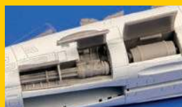
7453 F-14A Tomcat Port Side Cannon Installation
