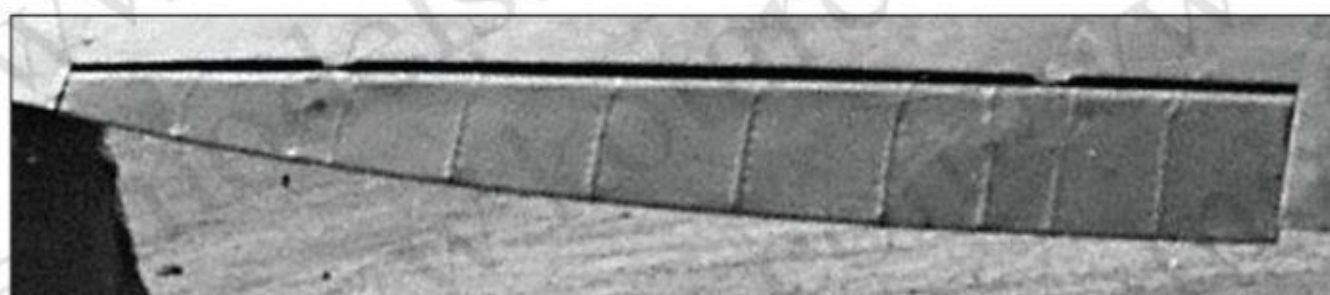
Aero Engines Ltd made port aileron from early-production Spitfire Mk.I (almost certainly K9910) showing the fabric stitching detail.
