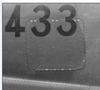
Accumulator door with raised rivets H10 from Spitfire Mk.Vb W3433.
