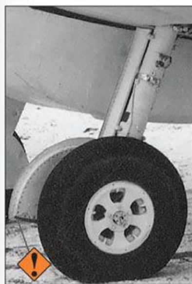
Undercarriage detail from late production Supermarine built Spitfire Mk.Vb AB344 photographed in January 1942. Note the 90 gallon "slipper" fuel tank and how the wheel, strut and door are painted the underside colour. The small flange at the bottom of the undercarriage door is a feature of Supermarine/Eastleigh built aircraft.
