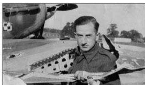
Edward Jaworski emphasizes the size of the hole in the wingtip. Unlike the rest of the wing, much of the internal wing tip structure was wooden, with most of the skin attached with screws.
