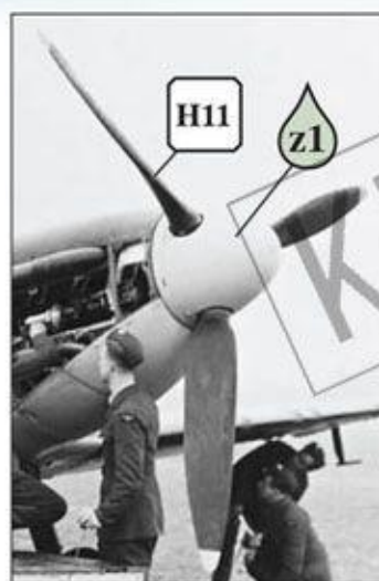
Rotol RX5/14 wooden propeller detail from an unidentified 65 Squadron CBAF built Spitfire Mk.IIa.
