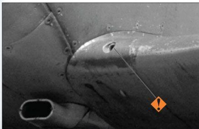
Camera gun port detail from Spitfire Mk.Vb BM202. Note the ill-fitting cowling panels.
