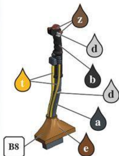
Offset control column with KG 13C hand grip
