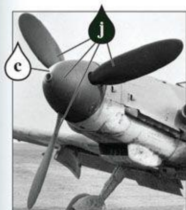
VDM 9-12159A propeller and spinner detail from late production Me 109K-4 335148. Theoretically the default spinner appearance was a sprayed white one third segment that bordered a propeller blade as here. Please see page 37 for a fuller discussion of spinner colour options. The 30mm Maschinenkanone 108 (MK 108 cannon) fired through the centre of the spinner and its exhaust gases vented through the bottom of the fuselage.
