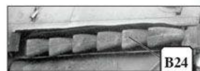
Starboard exhaust manifolds from the captured Bf 109K-4 seen on page 42. Note the weld lines.
