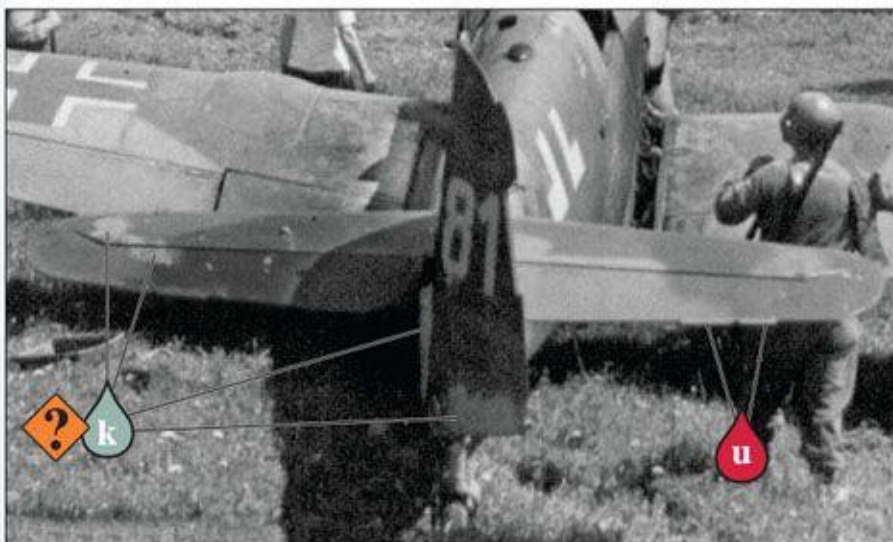
Tailplane detail from the unidentified mid-production Bf 109K-4 "White 81" seen on page 28. Note the various different unconfirmed upper surface camouflage colours and red painted trim tabs on the elevator.
